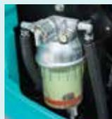
Pre fuel filter with built-in water separator
